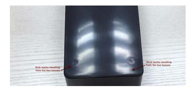
Changing injection molding parameters or component geometry can in some cases reduce sinking to an acceptable level as follows:
